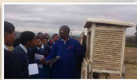
GEP technologist, Mr. M.S. Malinga taking students from Thembelihle High School through instruments kept in a Stevenson screen, and how an evaporation pan is used to estimate the rate of evaporation.
